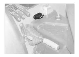
Screw out this regulator to increase lift lowering speed.
