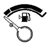
The green section shows how much fuel there is in the tank. The yellow fuel reserve light comes on when the lindicators light up in the red section.
