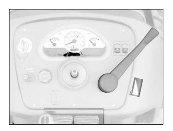
The throttle lever is located in the front right-hand side of the machine.
