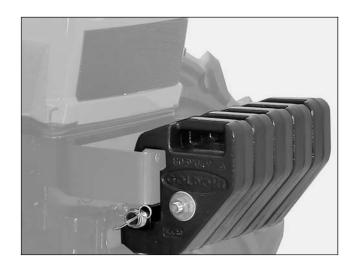
If heavy implements that could impair the stability of the machine are hitched, the optional plates can be used as front ballast.
