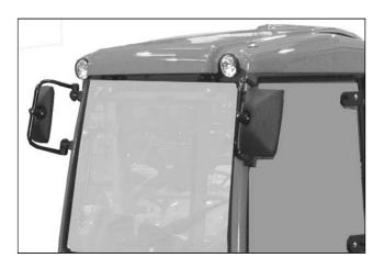
The rear view mirrors can be positioned in all directions and provide the user with excellent visibility from the driver's seat.
