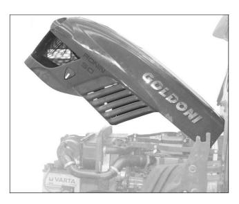
Once opene, the bonnet remains in the open position thanks to a gas spring Close the bonnet by lowering it until it completely engages with the lock
