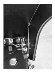
Use the rod to block the engine hood
