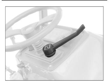
The throttle lever is located in the front right-hand side of the machine.
