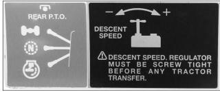
Screw out this regulator to increase lift lowering speed.
