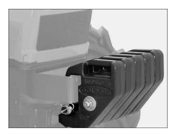
If heavy implements that could impair the stability of the machine are hitched, the optional plates can be used as front ballast.
