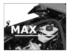
Top up the level of the cooling fluid when required:
