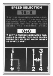
The machine has a **Dual Power** transmission, which provides 2 different gearshift modes selected with the GEARSHIFT MODE lever.
