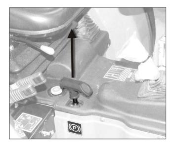
To disengage the parking brake:
