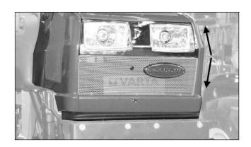
Once opene, the bonnet remains in the open position thanks to a gas spring Close the bonnet by lowering it until it completely engages with the lock
