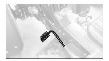
Transmits drive from the engine to the transmission.
