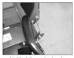
Use the rod to block the engine hood
