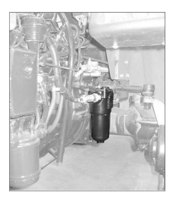
Replace the intermal cartridge of the transmission oil filter on the delivery:
