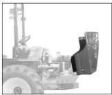
Use the rod to block the engine hood
