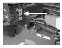
The metal plate is positioned in the interior of the right rear fender.
