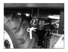
Ball joint with safety pins correctly mounted
