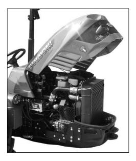
Use the rod to block the engine hood
