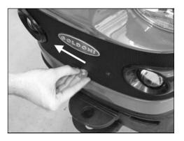
Use the ignition key and slide it to the left until the release of the lock
