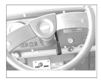
The throttle lever is located in the front right-hand side of the machine.
