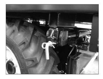
Ball joint with safety pins correctly mounted
