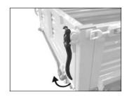
Unhook the two both side levers to release the rail
