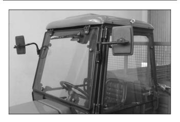
The rear view mirrors can be positioned in all directions and provide the user with excellent visibility from the driver's seat.
