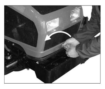
Use the appropriate tool in the accessory pack (6 mm Allen wrench) by turning it counterclockwise.
