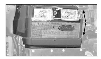
Once opene, the bonnet remains in the open position thanks to a gas spring
