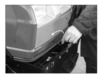
Use the appropriate tool in the accessory pack (6 mm Allen wrench) by turning it counterclockwise.
