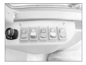
Select one of the electric fan's three speeds to change the amount of air that enters the cab.
