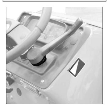
The throttle lever is located in the front right-hand side of the machine.
