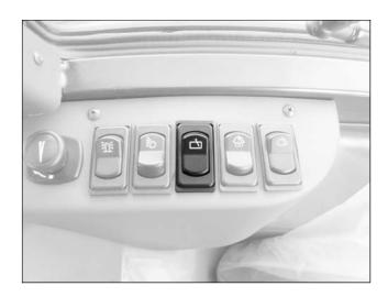
Operates when the ignition key is in the contact position. Press the switch in position one to operate the rear window wiper.
