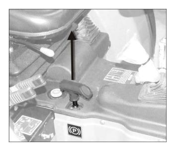
To disengage the parking brake:
