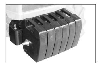
If heavy implements that could impair the stability of the machine are hitched, the optional plates can be used as front ballast.
