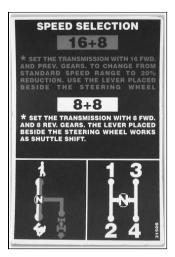
The machine has a **Dual Power** transmission, which provides 2 different gearshift modes selected with the GEARSHIFT MODE lever.
