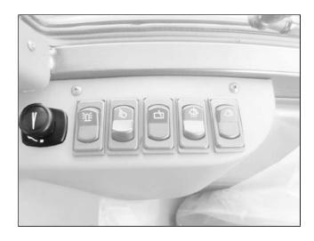
Select one of the electric fan's three speeds to change the amount of air that enters the cab.
