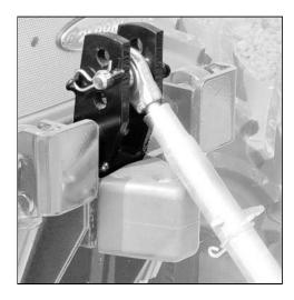
The top link linkage has three holes, which make the implement easier to hitch and set at the right angle. To adjust the top link, remove the split pin from the plug, remove the plug from the brackets, set the top link at the height of the required hole, then fit the plug and split pin back in position.
