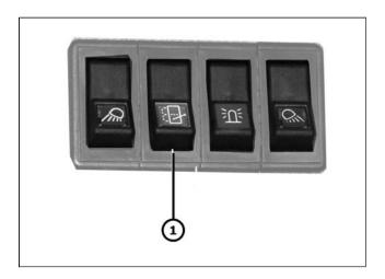
**NOTE:** The lower part of the button lights up when the light switch knob is turned to the side lights position (first position).
