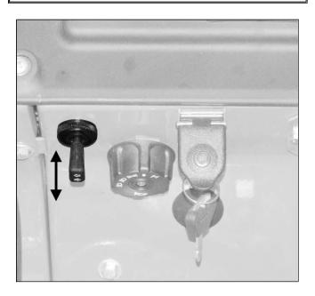
Push the switch down to flash the driving beams.
