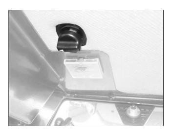
The cold air temperature can be regulated with the knob. Turn the knob to regulate the temperature. The lowest temperature in the cab is obtained by turning the knob in the clockwise direction (fully towards the right). Turn the knob fully to the left tp stop cold air from circulating around the cab.
