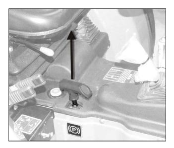
To disengage the parking brake:
