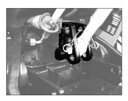
The top link's linkage has four holes to facilitate the hitching operation and ensure that the implement slants in the correct way.
