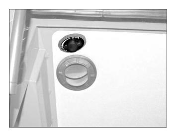
The hot air temperature can be regulated with the knob. Turn the knob to regulate the temperature. The highest temperature in the cab is obtained by turning the knob in the clockwise direction (fully towards the right). Turn the knob fully to the left tp stop hot air from circulating around the cab.
