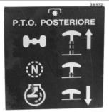
Having finished work, remember to move the PTO's mode selector lever back to the **Neutral (Idle)** position.
