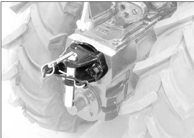
The machine can be equipped tow hook for the use of small trailers or the tanks of spraying equipment.
