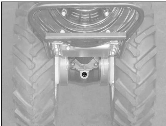
Replace the oil in the casing, which requires about 2 liters of fluid.
