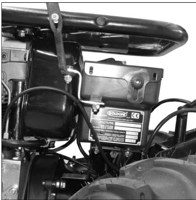
The metal plate is placed on top of the tools box.
