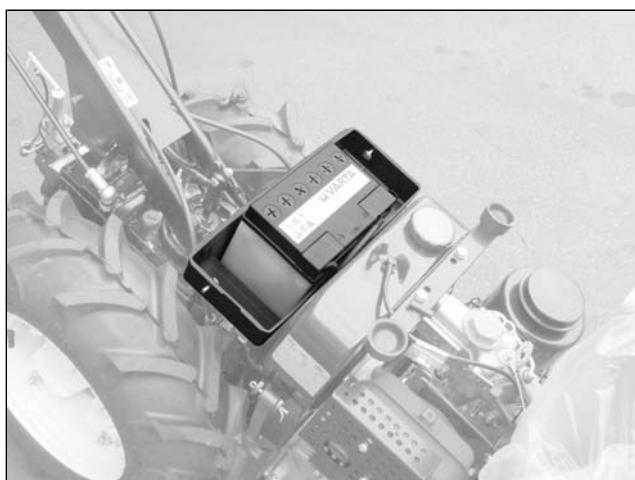
To access the battery open the bonnet and remove the protection removing the two side knobs (figure 1)
