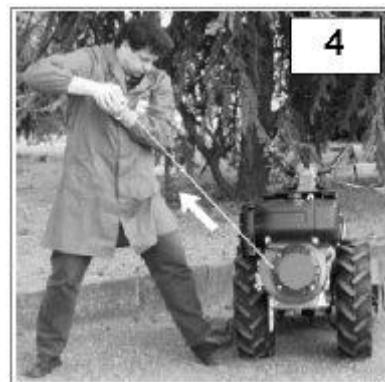
Hold the grip and pull the cord until compression is found (1). Completely rewind the cord (2) and then operate the decompression lever (3). Firmly pull the cord to start (4).
