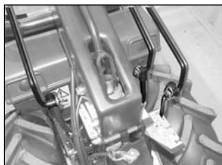
Fit the lever rod **①** **②** **③** in place and lock it with the split pins
