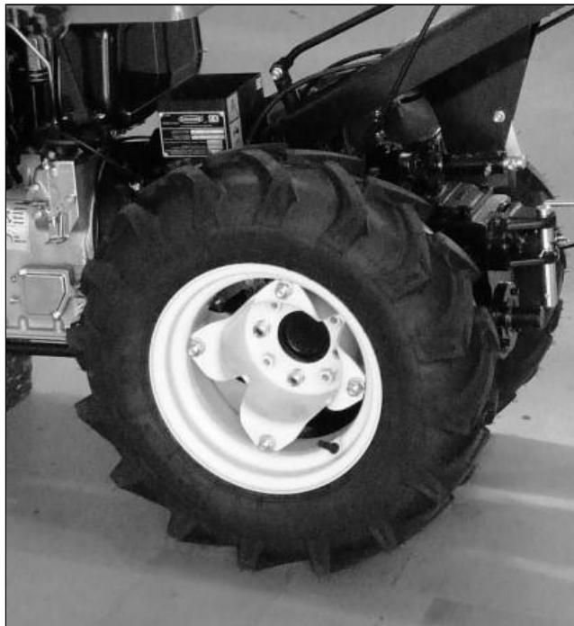
The wheel track can be changed by moving the wheel disc on his flange.
