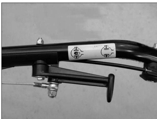
The tractor is equipped with a mechanical differential lock on both axles.
